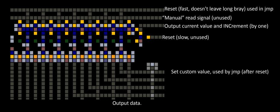
Data is read automatically when inc is sparked; this happens because near pscn there are DTEC(bray) that detect brown bray. To set manual read you can delete dtect and use read command. (and you can add dtect in counter) This counter is similar to the decfsz one. It uses the brown bray trick to change switch state.
