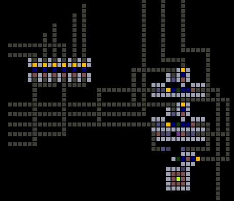
Small part of control unit designed to do something based on the Zflag: -first one increment IP if zflag is set: Switch is turned on by decfsz instruction (up) and zflag result goes from left to right. If zflag was set signal will be present and will also pass due to correct instruction.
