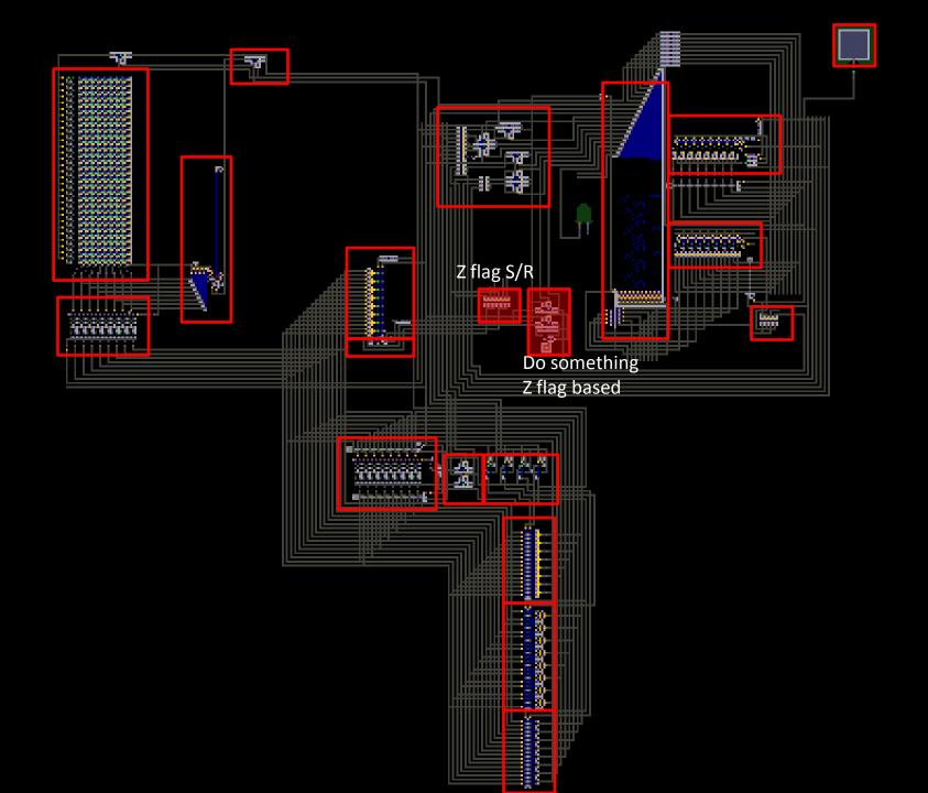
(half unused) signal joiner: it allows multiple input to single output without interference (something like a diode array) It was intended to be used to set and reset Z flag from different commands
