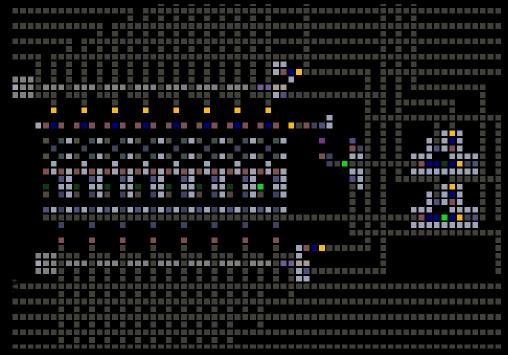
The main register is similar to the memory register. As extra it has two ports (on right) that select the mode of operation: read or write (1 bit). There is the execute/enable bit (that will read or write).
