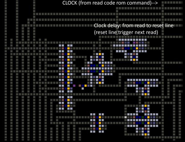
From code ROM (instructions) Some wires are directly connected to the command bus, others pass through the control unit.
