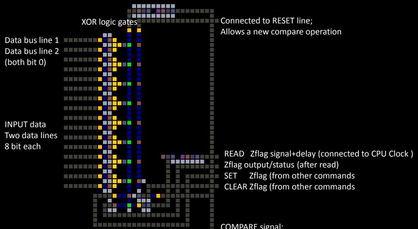
READ Zflag has a delay so that it is read AFTER all computations are done; in this way we read it after it has been set/cleared. COMPARE signal: -reset Z flag (SWCH down) -spark ray up If all swch are ON data is equal and ray gows down and turn on the last SWCH If data is different it pass in the logic gate and enable the NSCN that turn off a SWCH so Z flag will not be sparked
